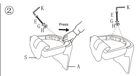
First install the central screw and tighten it to 70%, then install the screws on both sides and tighten them to 80%
