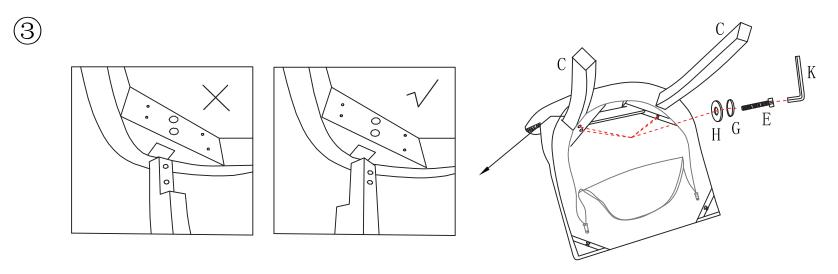
Tighten all the screws to 80% of maximum tightness
