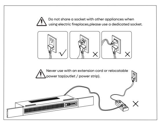
A 15 AMP circuit is required to operate this appliance. If the breaker trips when the appliance is running, you may need to move the appliance to another location or unplug other appliances that are on the same circuit.
