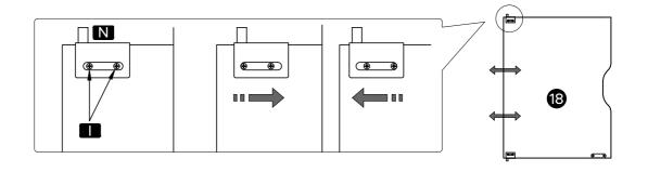
$\ensuremath{\mathbb{X}}$  Please adjust the pivot positon slightly to make sure the gap between both doors are aligned
