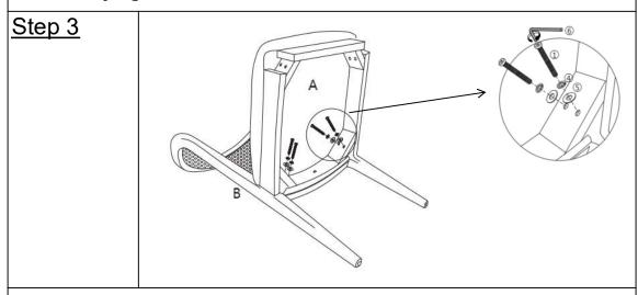
Lock the corner four mounting positions and attach them using Bolts(1), Spring Washers(4) and Washers(5) with Allen Wrench(6), as shown on the picture above.
