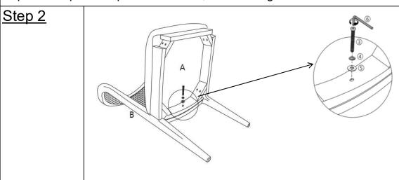
Place the Back with Legs(B) on a clean, non-marring surface. Align the mounting positions on the Seat(A) to the mountings on the Back with Legs(B).
