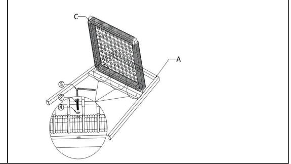
Open the carton and place all the parts onto a clean, non-marring surface. Attach the Seat(C) to the Right Armrest/Leg(A) using Bolts (②) and Washers (④) with the Allen Wrench (⑤) as shown above. Do not fully tighten the Bolts.
