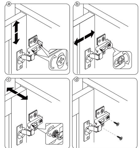
NOTE: If the doors are uneven or there is a gap in the middle, loosen or tighten the screw on the door hinge until they are sitting flush.
