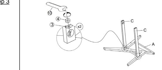
Attached Stretcher (C) to Right Arm (A) by using the Half Moon Washer (③) ,Nut (④) and Open wrench (⑩) as pictured above.
