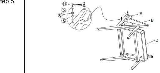
Attached Back Cushion (E) to Left Arm (B) by using the Bolt (5), Spring Washer (6), Flat Washer(8) and Allen Wrench (11) as pictured above.
