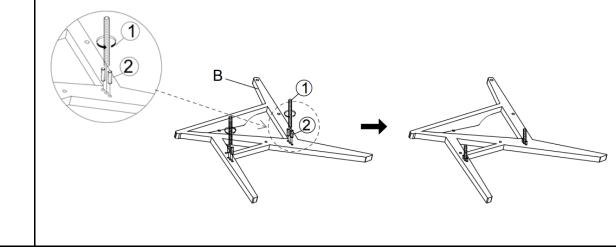
Install the Full Thread Screw (1) and Wood Dowel (2) on the Left Arm (B) ,as pictured above.
