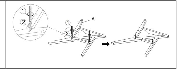
Install the Full Thread Screw (1) and Wood Dowel (2) on the Right Arm (A), as pictured above.
