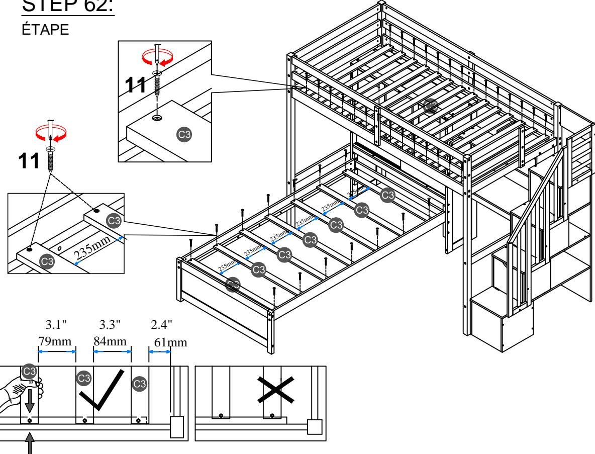
**NOTE:** Please make sure the bed slats close to the side rail before locking the screws to avoid breakage. This step is required for both the left and right sides. Moreover, please do not lock the screws of the bed slats at the outermost edge to avoid damaging.
