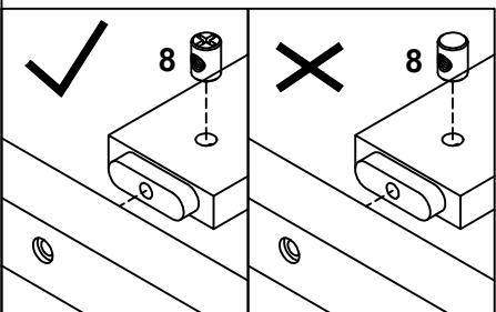
Note: Part 8 will face up with the "x" mark on it, otherwise it cannot be tightened
