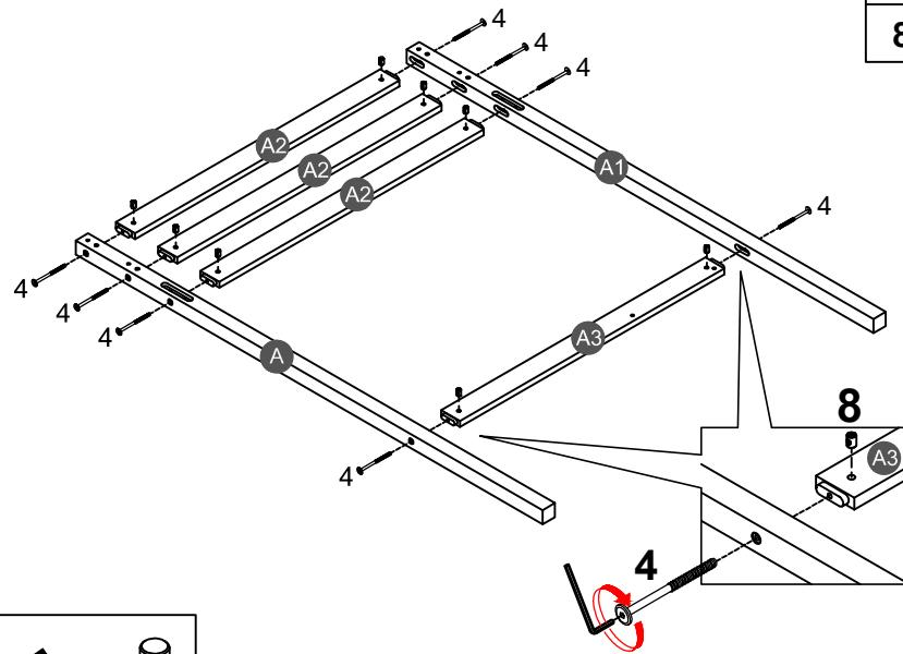
Note: Part 8 will face up with the "x" mark on it, otherwise it cannot be tightened
