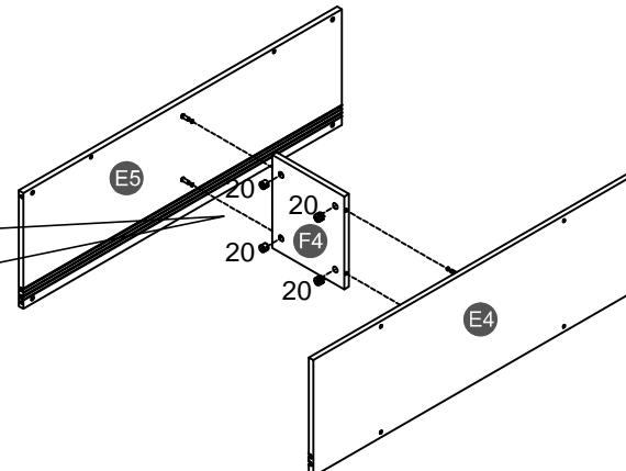
Note: Place hardware #20 with the "X" face outward, and make sure that the arrowhead is upward. Then, place hardware #20 into the hole of hardware #19 and tighten it clockwise with a hand screwdriver. (Please do NOT use an electric screwdriver.)
