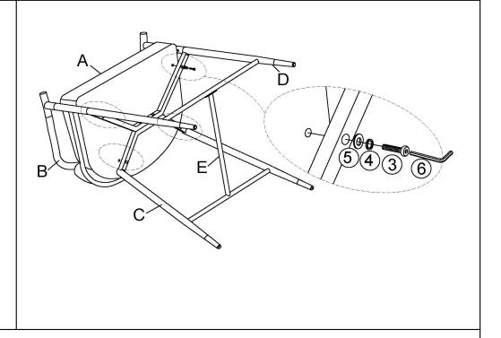
Using Bolt(③), Spring Washer(④), Washing Ring(⑤) with Allen Key(⑥) to fix Seat(A), Back Leg(C) and Front Leg(D).
