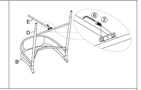
Attach the Rail(E) to middle of Front Leg(D) using Bolt(②) with Allen Key(⑥).
