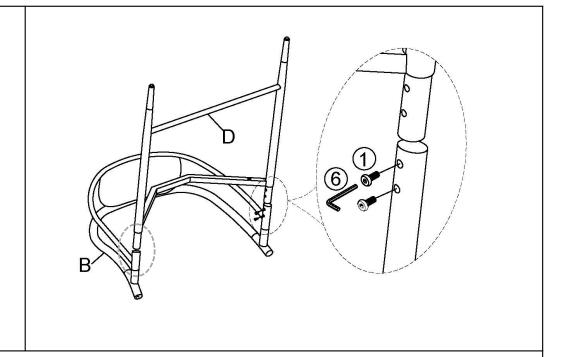
Attach the Front Leg(D) to the bottom of Backrest(B) using Bolt(1) with Allen Key(6).
