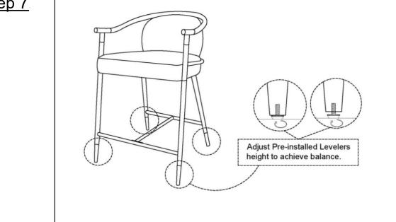
With assistance from your adult partner, stand the Counter Stool up. Adjust the Pre-installed Levelers at the bottom of Back Leg(C) and Front Leg (D) until the Counter Stool is level with the ground.
