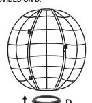
4. INSERT PART E INTO THE TOP OF THE ATTACHMENT (A+B+C). ENSURE THE CONNECTIVE TOP OF THE ATTACHMENT GETS FIXED IN THE GROOVE PROVIDED ON E.
