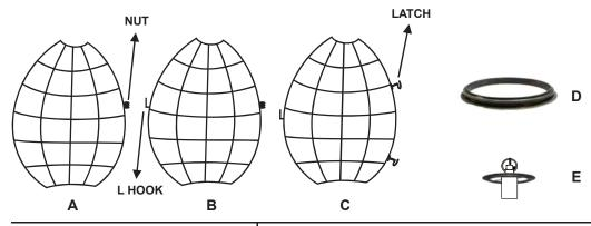
1 . INSERT THE L HOOK, PROVIDED ON B, INTO THE NUT, PROVIDED ON A .
