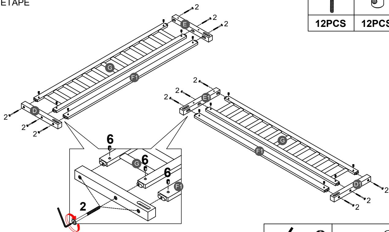
Note: Part 6 will face up with the "x" mark on it, otherwise it cannot be tightened
