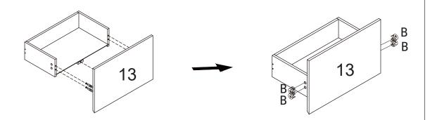
Need to rotate and tighten B
