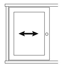
LEFT AND RIGHT Use screw to adjust the gaps at left and right of the door.
