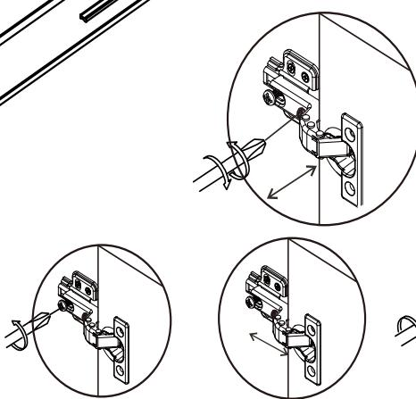
This is used to adjust the door panel in the front and back direction: Loosen the screw first, and then tighten screw after adjusting the door panel to the proper position.
