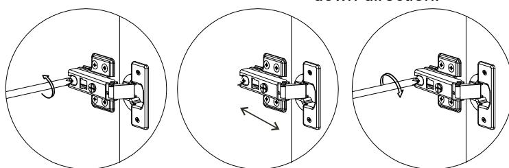
This is used to adjust the door panel in the front and back
