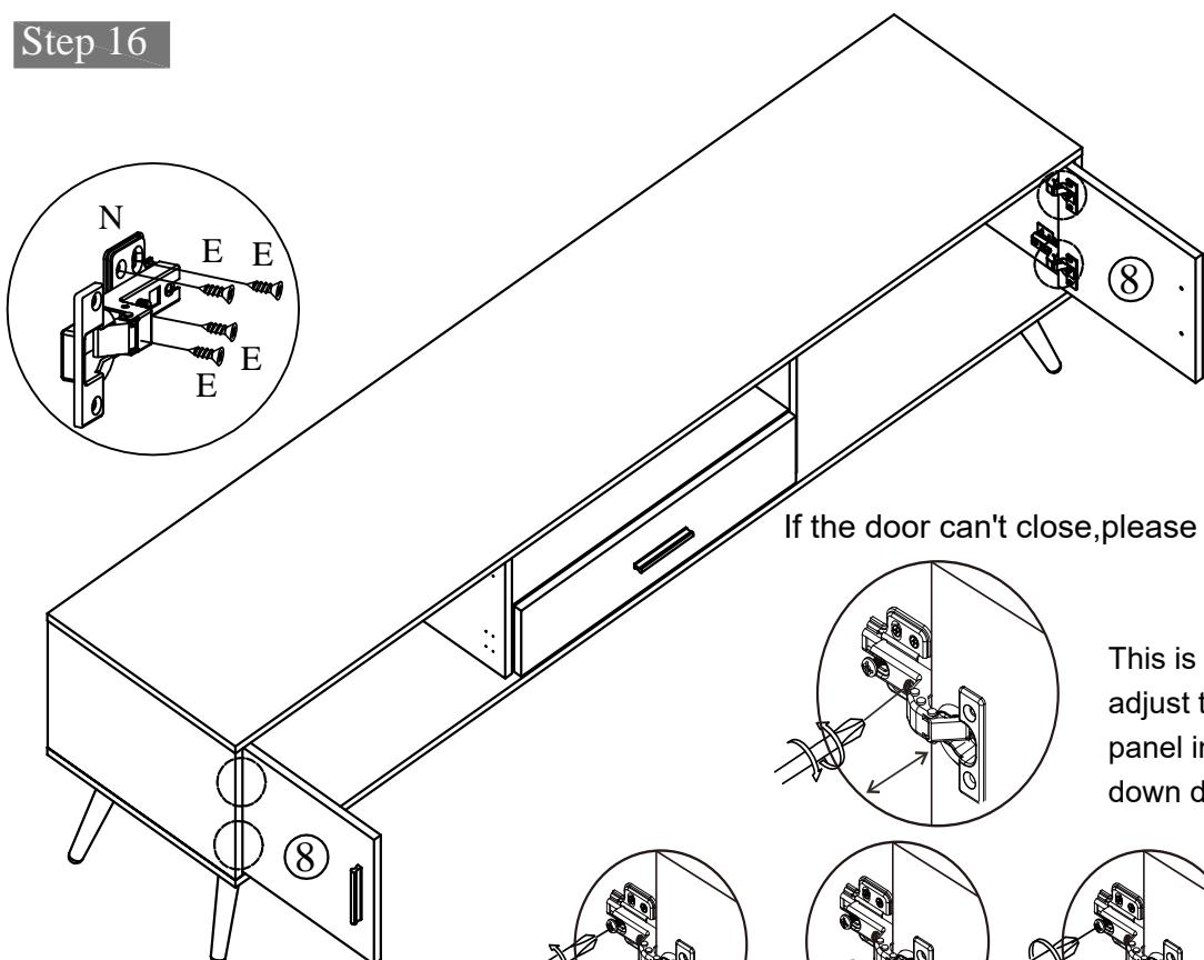
This is used to adjust the door panel in the up and down direction.
