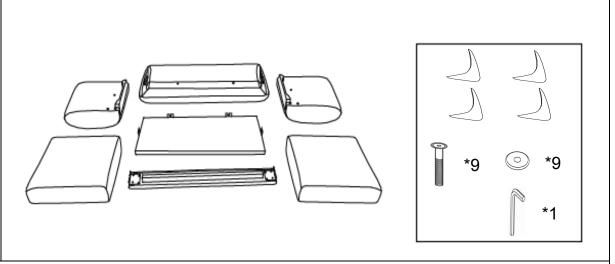
Position the Backrest(A),Left Armrest(B),Right Armrest(C),Seat Cushion(D),Leg(E),Seat Board (F) and Frontal Seat Board(G) on a clean,non-marring surface as shown.
