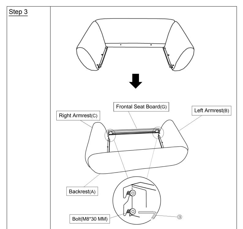
Place the Frontal Seat Board (G) as shown in the above pictures in front of the semi-sofa from step 2,hang the Brackets on the Bolts(M8\*30 MM) found on the Armrests (B&C).
