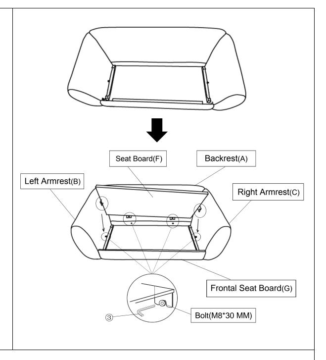
Using the Allen Wrench ( ) and turning Counter-Clockwise, loosen all the Bolts(M8\*30 MM) which are pre-assembled on the Backrest (A) and Armrests (B&C) about 3 threads out to make a small gap in which to fit the metal brackets.
