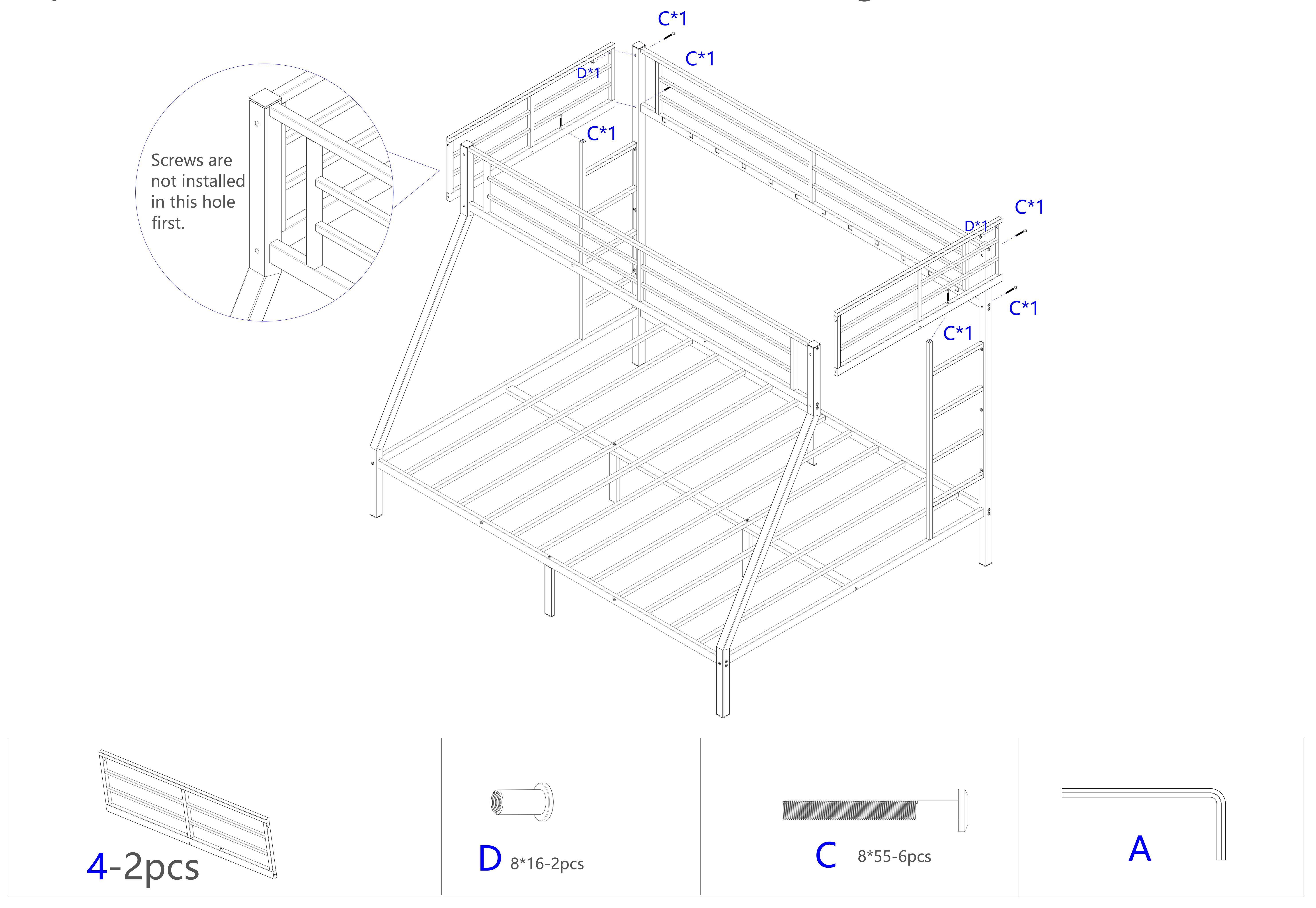
Step 9: Use hardware A and C to connect #8 together.
