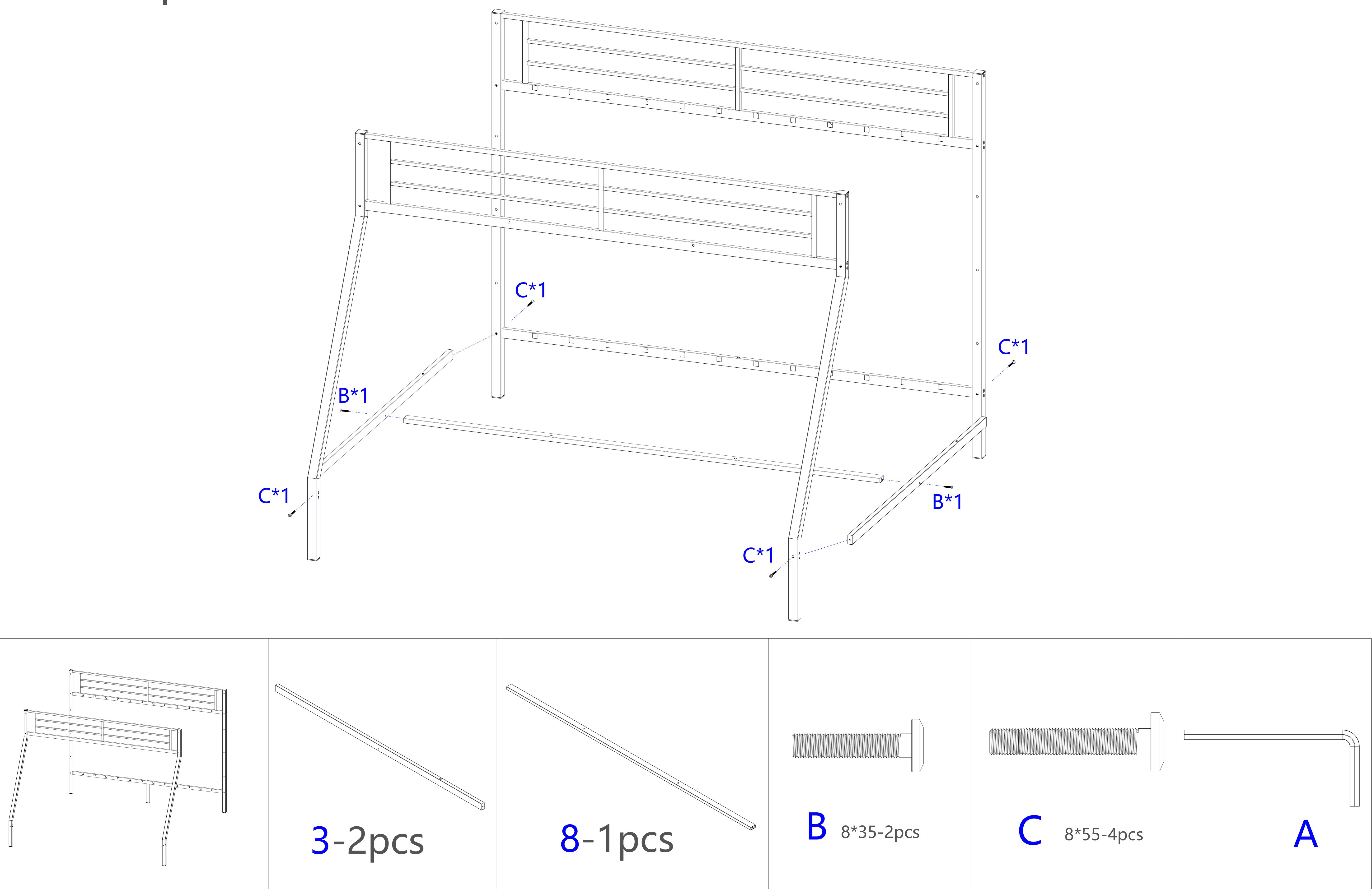
Step 4: Use #9 and #10 to insert the corresponding square hole of #6.
