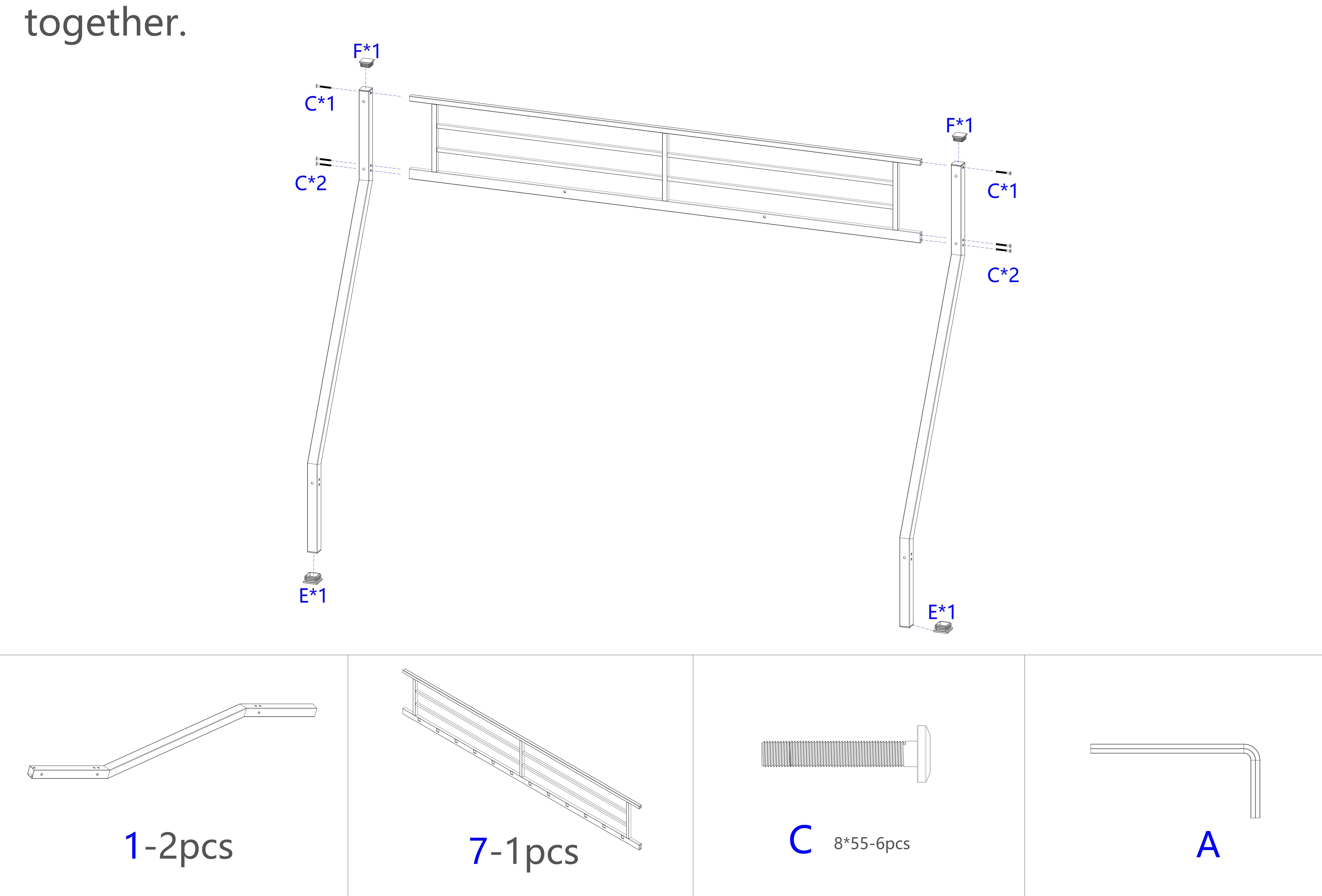
Step 3: Use hardware A, C, and B to connect #3 and #8 to the front part.
