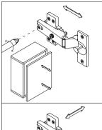
If the hinge holes are notaligned, you can tryadjusting the front and rear hinges.
