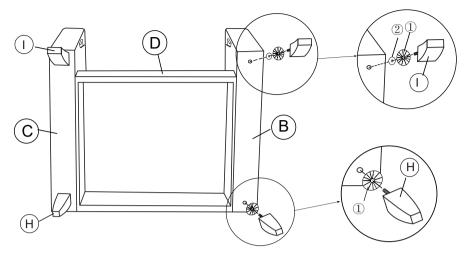
Place one Plastic Washer(1) and on the Front Leg(H) screw,then insert screw into the mounting hole at the corner of the chair. Tighten by turning the leg clockwise as shown. Repeat the same steps to install the other Front Leg(H).
