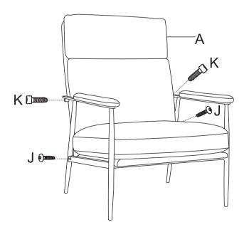
STEP 5 Please 100% tighten all Allen Bolts (G,H,I) completely by using Allen Wrench (L) . After initial assembly, the product may acclimate to its new environment. Please ensure all screws are still securely tightened.
