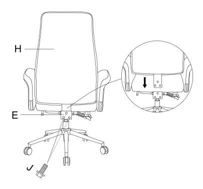
STEP 8 In this step please make sure the chair is flat and all bolts are installed, then finally 100% tighten all bolts.
