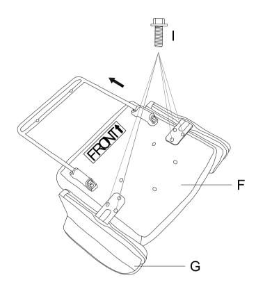
STEP 4 Attach the Seat plate(E) to the seat(F) by using Allen bolt (I) and Allen Wrench (N).
