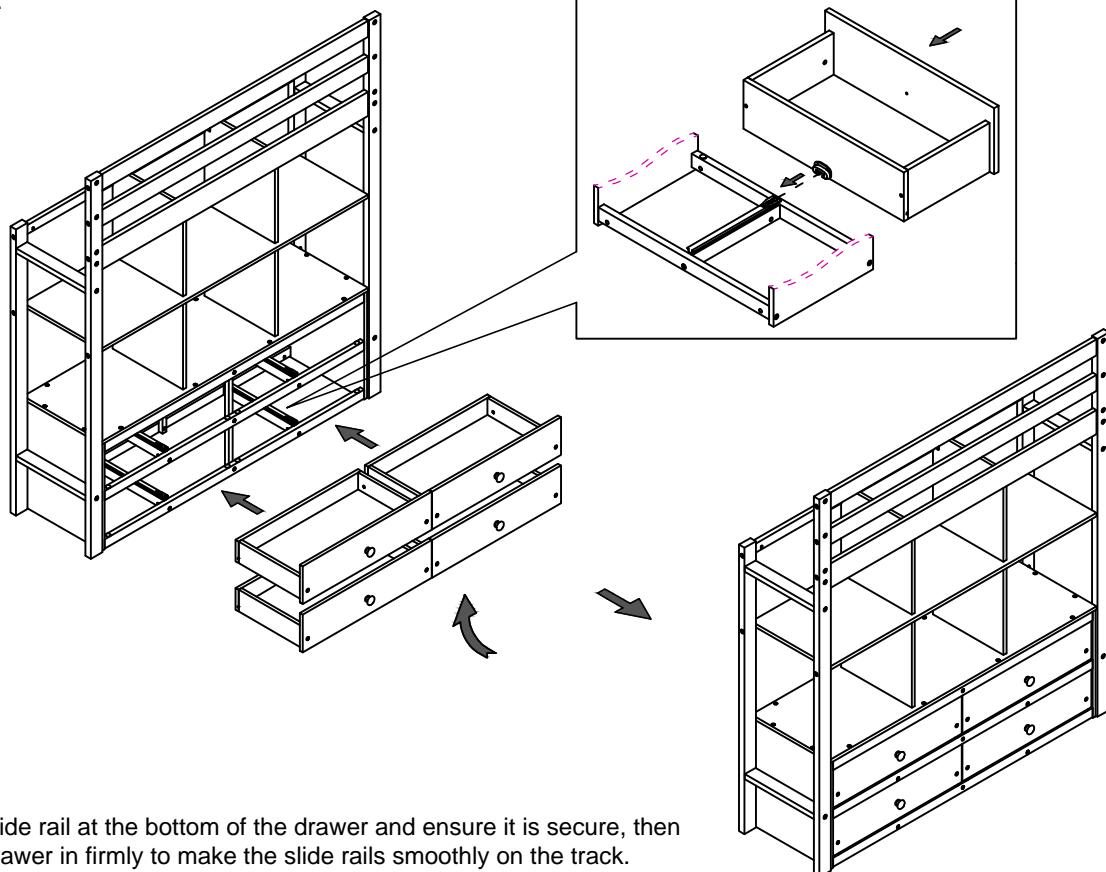
Align the slide rail at the bottom of the drawer and ensure it is secure, then push the drawer in firmly to make the slide rails smoothly on the track.
