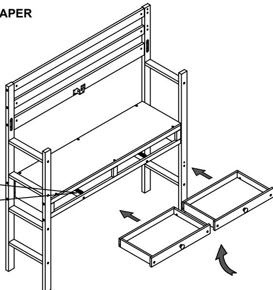
Align the slide rail at the bottom of the drawer and ensure it is secure, then push the drawer in firmly to make the slide rails smoothly on the track.
