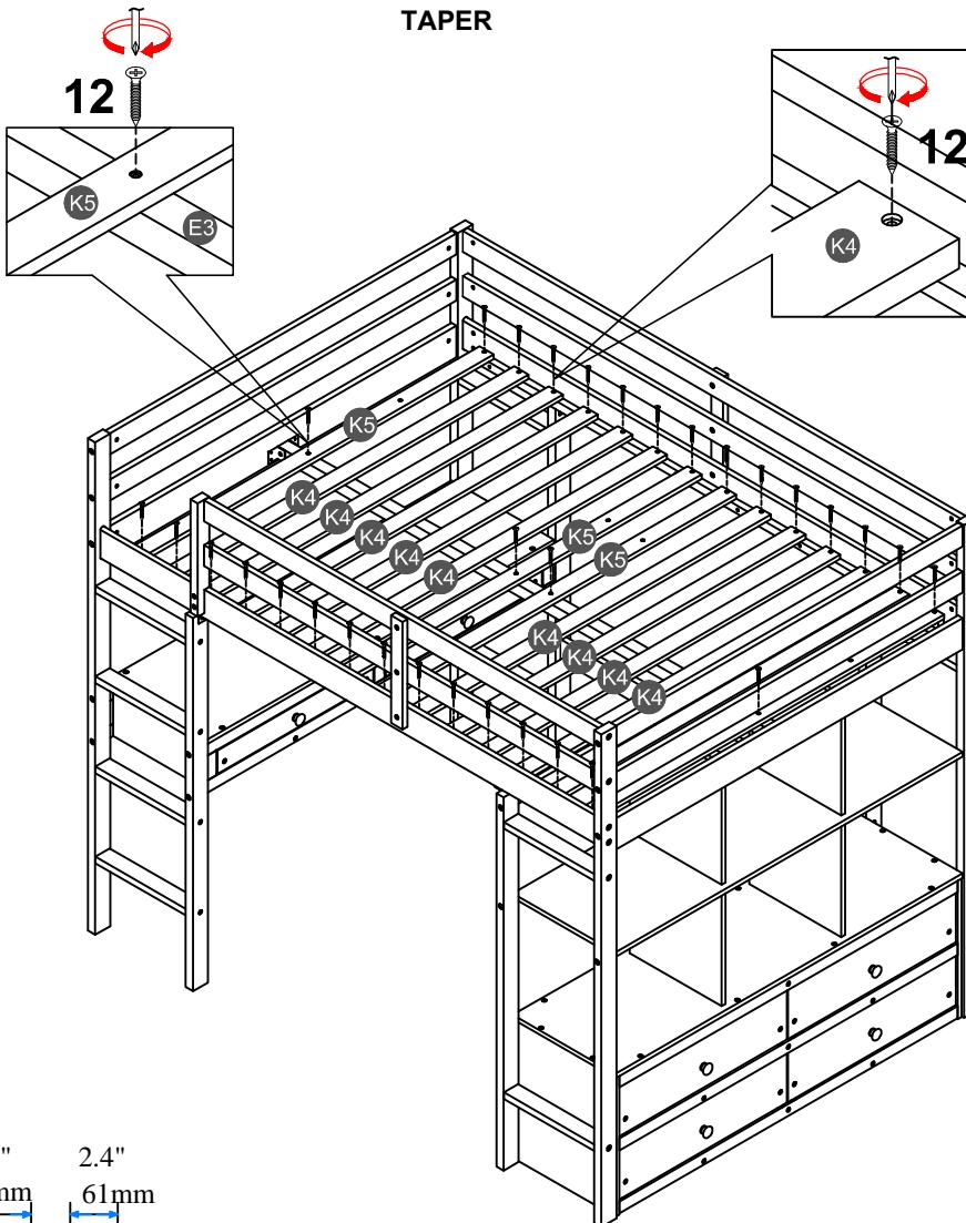
**NOTE:** Please make sure the bed slats close to the side rail before locking the screws to avoid breakage. This step is required for both the left and right sides. Moreover, please do not lock the screws of the bed slats at the outermost edge to avoid damaging.
