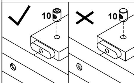
Note: Part 10 will face up with the "x" mark on it, otherwise it cannot be tightened
