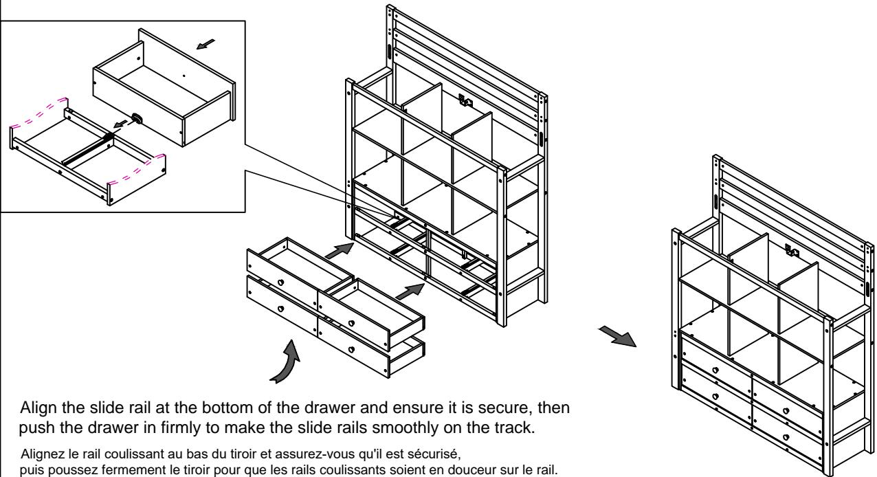
Align the slide rail at the bottom of the drawer and ensure it is secure, then push the drawer in firmly to make the slide rails smoothly on the track.
