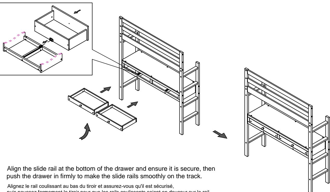
Align the slide rail at the bottom of the drawer and ensure it is secure, then push the drawer in firmly to make the slide rails smoothly on the track.
