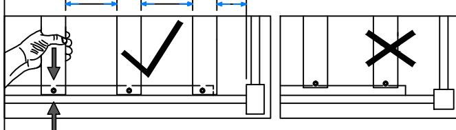
**NOTE:** Please make sure the bed slats close to the side rail before locking the screws to avoid breakage. This step is required for both the left and right sides. Moreover, please do not lock the screws of the bed slats at the outermost edge to avoid damaging.
