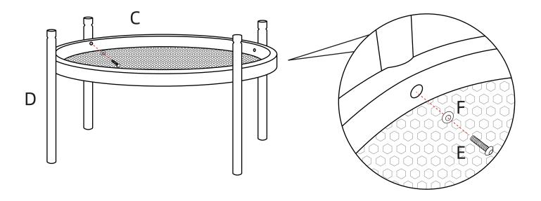
1. Invert C and 4 D wires, as shown in the above figure, using E&F installation and fixation.
