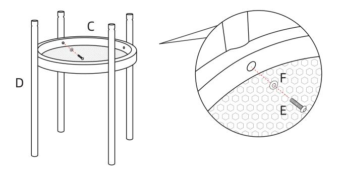
1. Invert C and 4 D wires, as shown in the above figure, using E&F installation and fixation.
