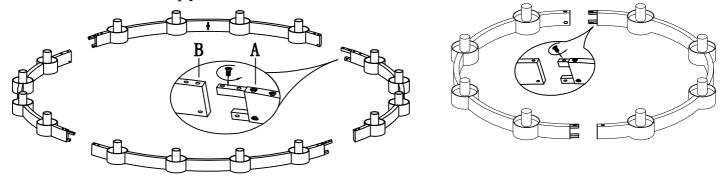
If the circular hole position of the screw installation cannot be aligned with accessory B, please loosen the screw of model A, insert the accessory of model B again and align the circular hole position. then tighten the screw.
