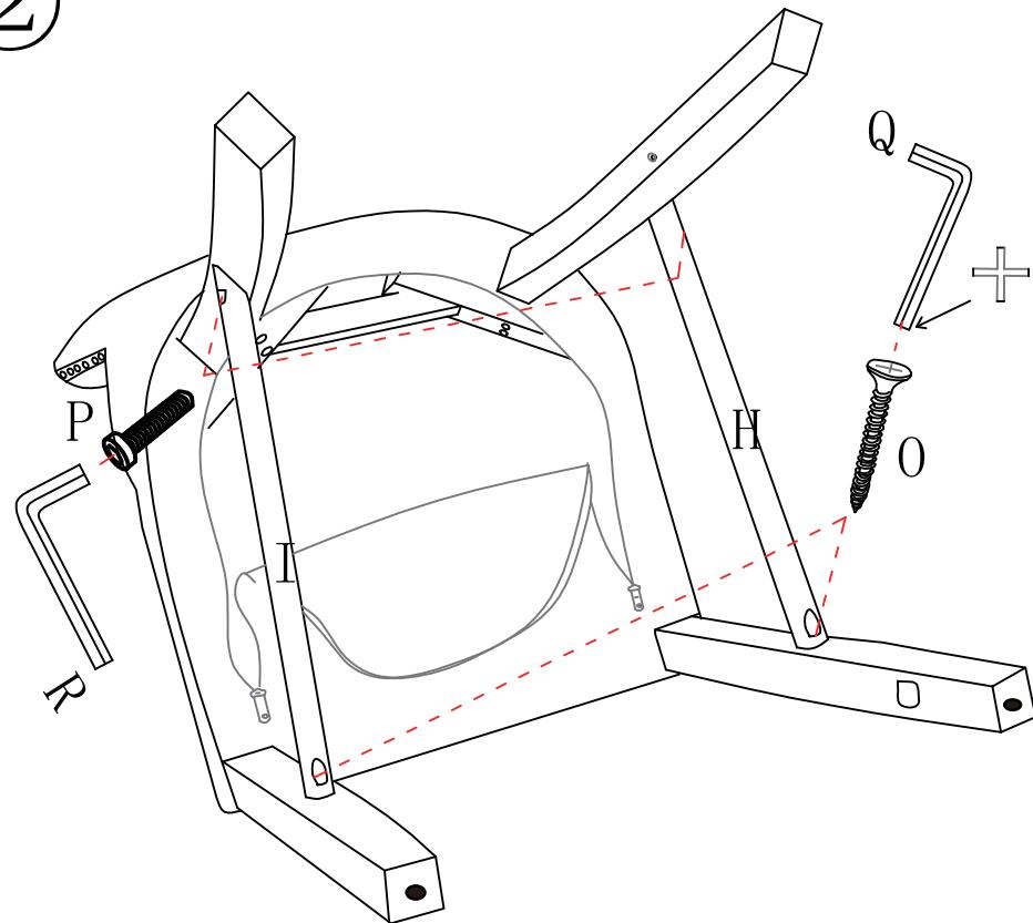
Caution: The bars H and I should be in horizontal position after installation. If not, the most possible reason is the rear feet were not installed correctly. Please check and swap the left and right rear feet.
