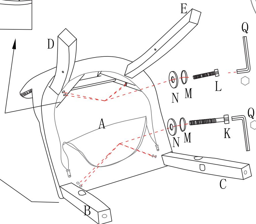
3. Tighten all the screws to 80% of maximum tightness.
