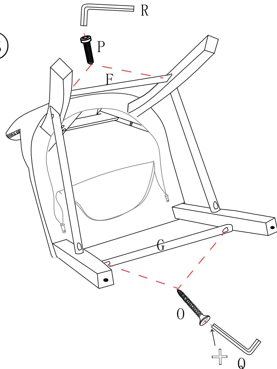
Tighten all the screws to 80% of maximum tightness.
