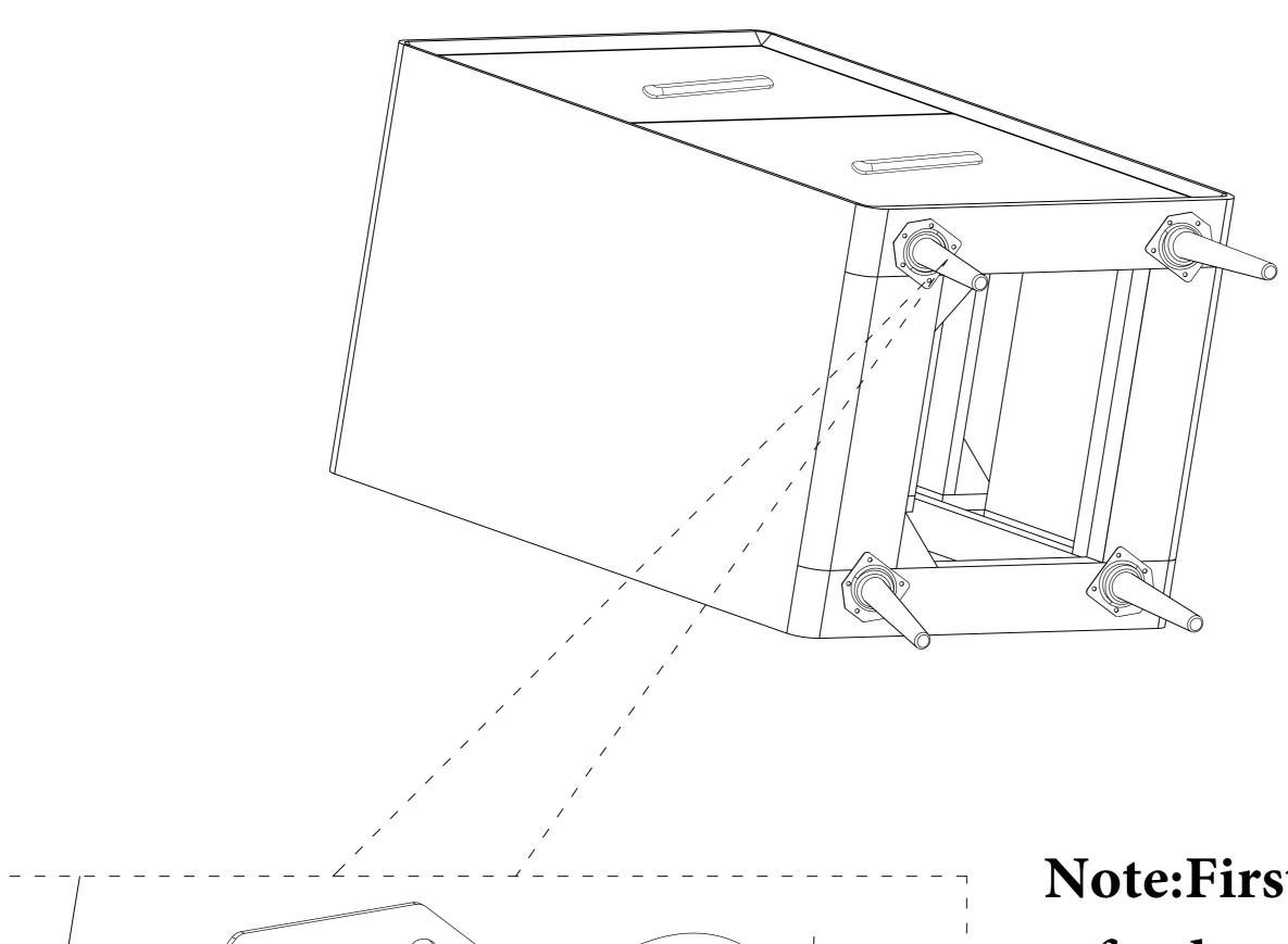
Note: First put the product down in a safe place, according to the direction indicated in the enlarged picture to tighten the foot and hardware hole button!
