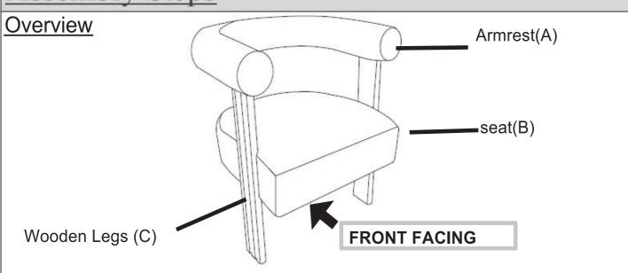
This chair has multiple parts and may require up to 30 minutes to assemble. To give you an overview of the chair parts, the above picture is provided to help you put the various parts into perspective. Please read through the instructions below to familiarise yourself with the parts and steps before assembly.
