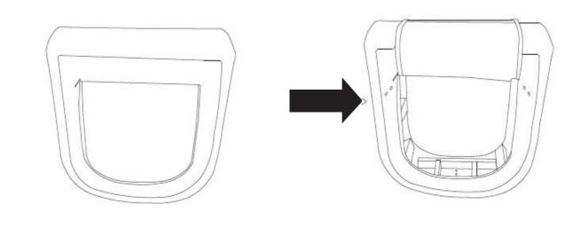
Place the bottom of the Seat (A) upwads, then unzip to open, to reveal the screw holes inside the seat frame as shown
