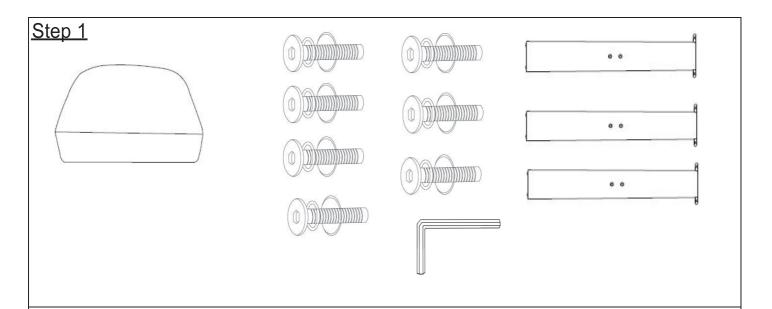
Place the Seat(B),and Bolt M8X40mm(1),and Spring Washer(3),and Flat washer(4),and three Legs(C)on a clean, non-marring surface. Before this, please string the Spring Washer(3), and the Flat washer(4) onto the Bolt M8X40mm(1), with the Spring Washer(3) in the middle as shown.
