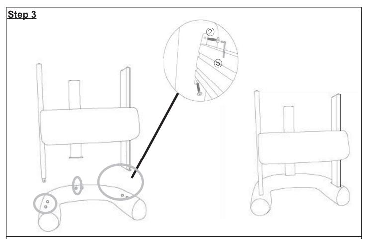
Put the armrest upside down.Please align the assembled foot and seat products, take out armrest (A). Align the holes under the armrest with the holes on the iron plate at the top of the foot, and use a Allen Wrench(⑤) to insert the Bolt M8X25mm(②) into the aligned hole and tighten it.
