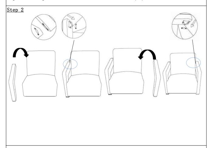
Straighten the assembled backrest and seat, take out the Left leg(C) and right leg(D), and insert the leg into the plug-ins at the left and right ends of the backrest(A).
