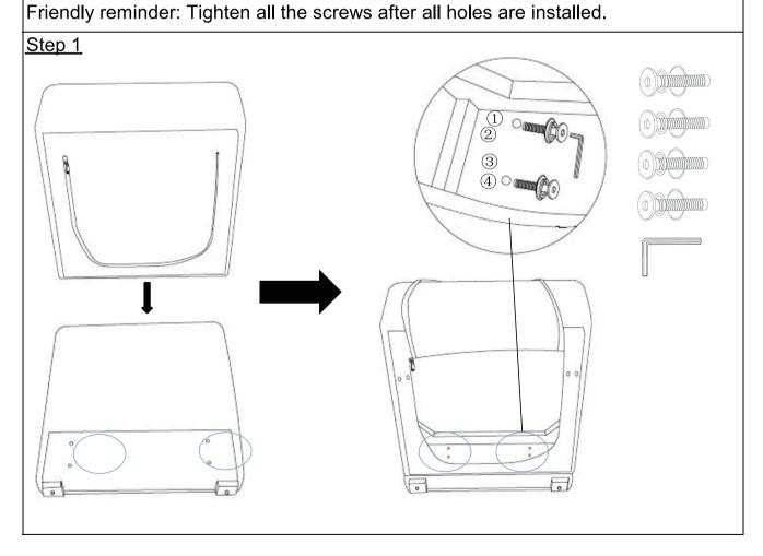
Take out the backrest(A) and seat surface (B) first, align the holes on the seat(B) with the holes on the backrest(A). Unzip the non-woven zipper at the bottom of the seat to expose the entire bottom, make sure the holes on the seat and backrest are aligned, then tighten the screw with the Allen Wrench(4) socket.
