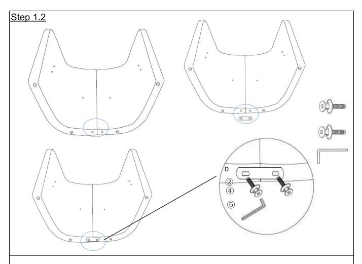
After the backrest is assembled, please take out Sheet Iron(D) and align it with the holes. Use Bolt M8X20mm(2) and Flat Washer(4) and tighten it with the Allen Wrench(5). The purpose of tightening the iron sheet screw in this step is to strengthen the firmness of the backrest assembly on both sides.
