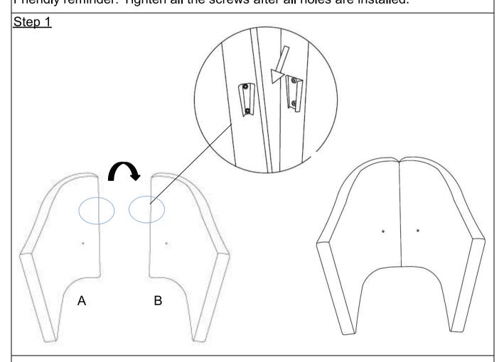
Take out the Left-Backrest(A) and Right-Backrest(B). There are latches at the bottom of the ends of the backrests. Please insert the left and right latches to close them. Insert A into B as shown
