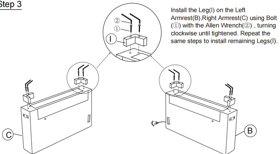
Install the Leg(I) on the Left Armrest(B),Right Armrest(C) using Bolt (①) with the Allen Wrench(②) , turning clockwise until tightened. Repeat the same steps to install remaining Legs(I).
