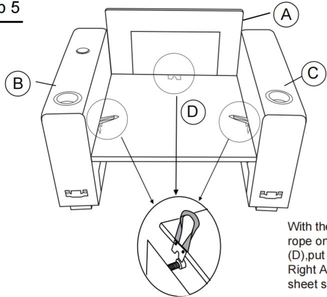
With the assistance of your partner, lift the rope on the two sides of the Seat Panel (D), put it down between Left Armrest(B) and Right Armrest(C) then make all u-shaped iron sheet stuck bolts as shown.
