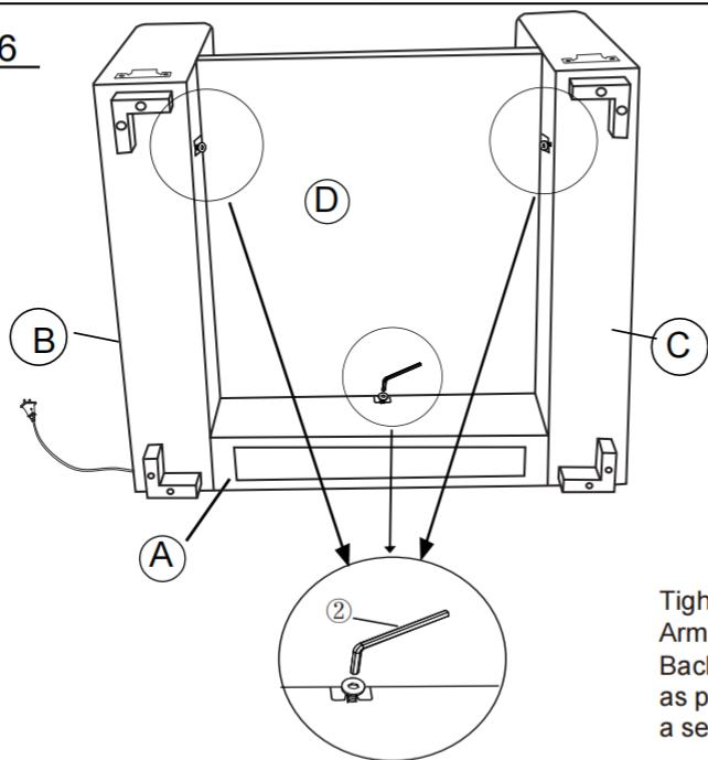
Tighten the Bolts in the bottom of Left Armrest(B) ,Right Armrest(C) and Backrest(A) by Allen Wrench(②) as pictured. Tighten the Bolts fully in a sequential manner.
