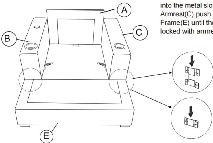
Insert the metal device on Front Seat Frame(E) into the metal slot on Left Armrest(B) and Right Armrest(C),push down the Front Seat Frame(E) until the Front Seat Frame(E) is fully locked with armrests.
