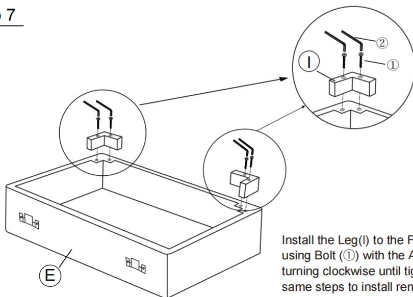
Install the Leg(I) to the Front Seat Frame(E) using Bolt (①) with the Allen Wrench(②) , turning clockwise until tightened. Repeat the same steps to install remaining Legs(I).
