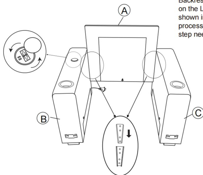
Slide the Tapered Connectors on the Backrest(A) into the Tapered Connectors on the Left Armrest(B) until locked as shown in the picture. Repeat the same process with the Right Armrest(C).This step need two persons to finish.
