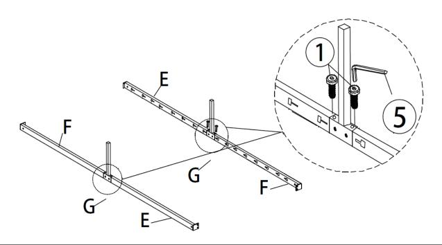
Align the mounting positions of Rail Support Leg(G) to Side Rail(E&F). Attach Rail Support Leg(G) to Side Rail(E&F) using Bolt(1) with Allen Key(5).
