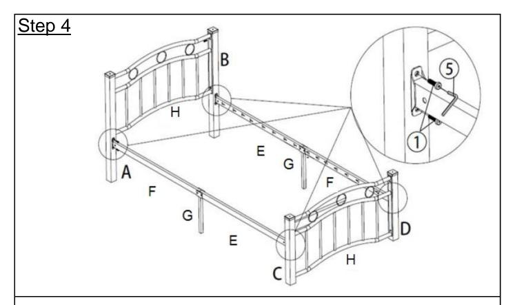
Turn over the assembled rails. Attach Side Rail frame(E&F&G) to Headboard/Footboard(H) using Bolt(1) with Allen Key(5).
