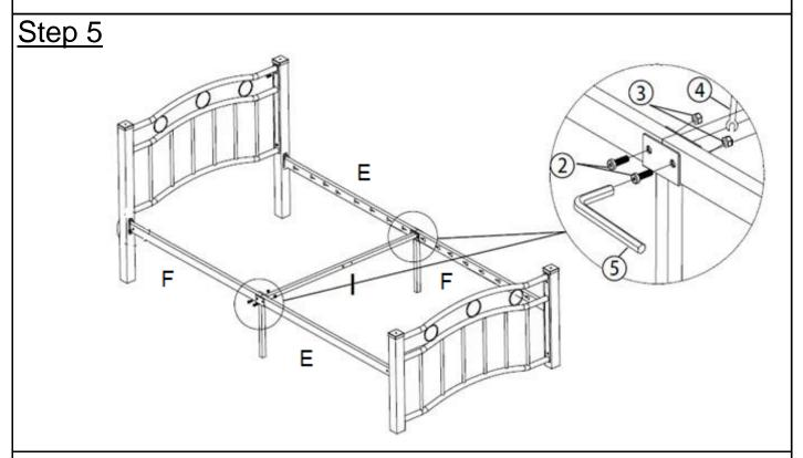
Attach Cross Center Support Rail(I) to the Rail(E&F) using Blot(2) and Nut(3) with Allen Key(5) and Wrench(4).
