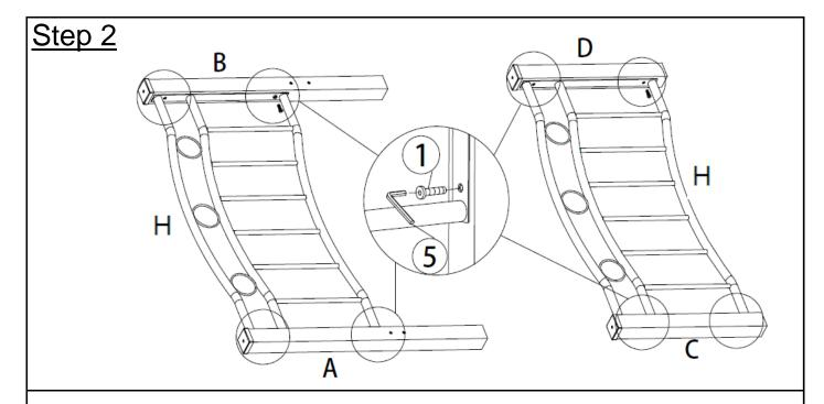
Attach Left Headboard Foot(A) and Right Headboard Foot(B) to Headboard/Footboard(H) using Bolt(1) with Allen Key(5), as shown in above picture.
