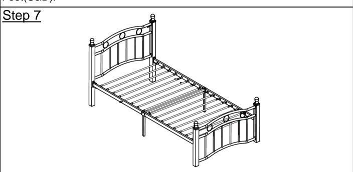
Now, fully and securely, tighten all nuts, at all joints. Inspect it and make sure all parts are adequately connected. Your bed is ready for use.
