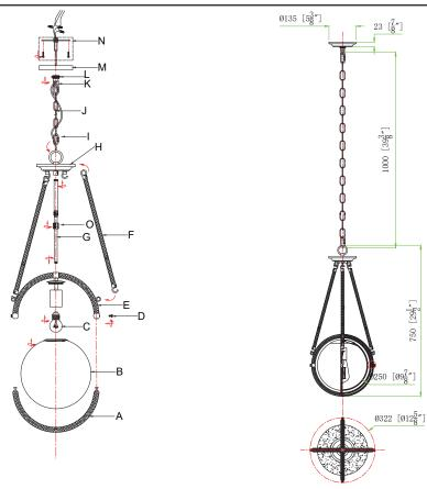
A: Bottom frame B: Glass shade C: A19 E26 bulb(Not Included) D: Screws
