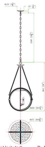
A: Bottom frame B: Glass shade C: B10 E12 bulb(Not Included) D: Plate
