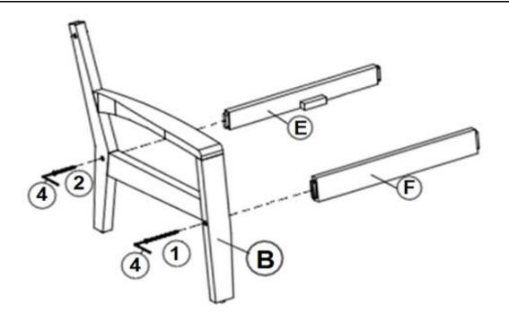
Place Left Arm Panel (B) stand up as shown in picture onto a clean, soft surface to avoid any scratches or damages to the product.
