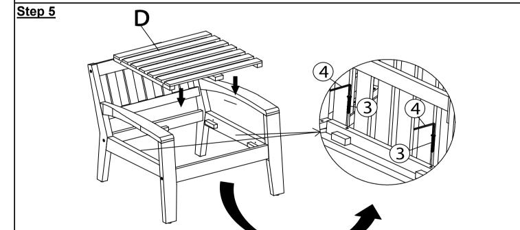
Attach the Seat Panel (D) onto the Armchair as shown in picture above.
