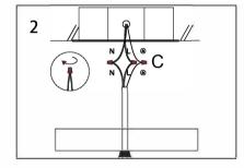
3. Install the canopy to the bracket with cap nuts D.
