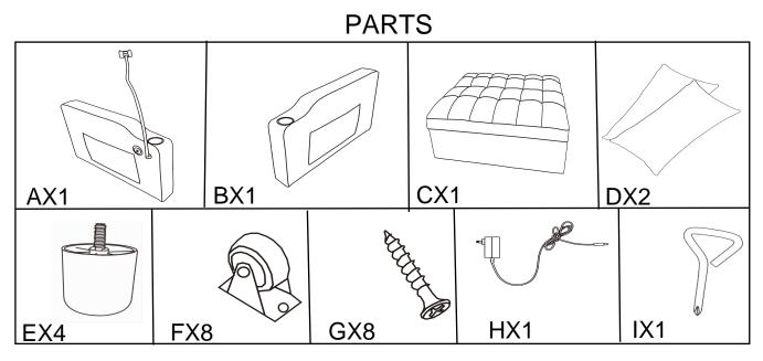
Step1:Open the box, fix the wheel (F) in its position with self tapping screws (G), and then rotate the mounting feet (E) to ensure that all feet are securely installed.
