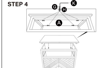
Place the top panel and secure with screws and washers as shown.
