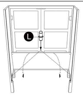
Insert the dowel pins and unfold the bottom panel.
