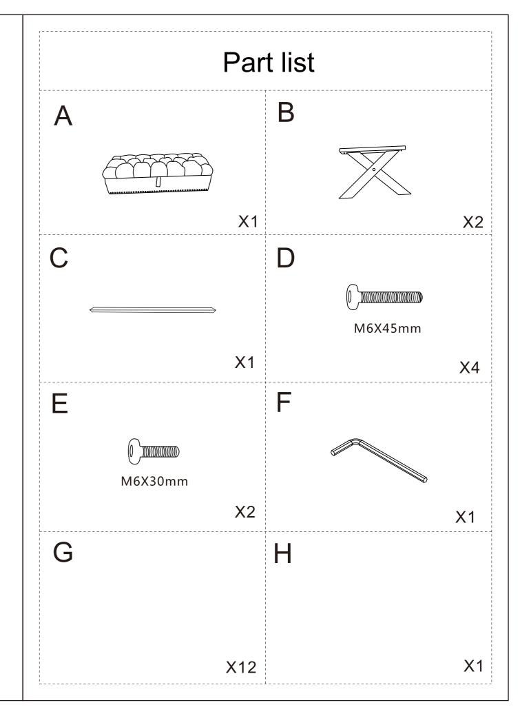
Use bolts (E) to fix the crossbeam (C) in the middle
