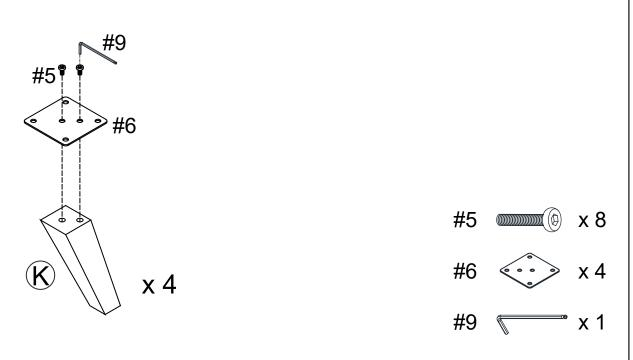
Step 10. Attach assembed legs (part K) to bottom (part E) using short bolts (part #5) and allen wrench (part #9).
