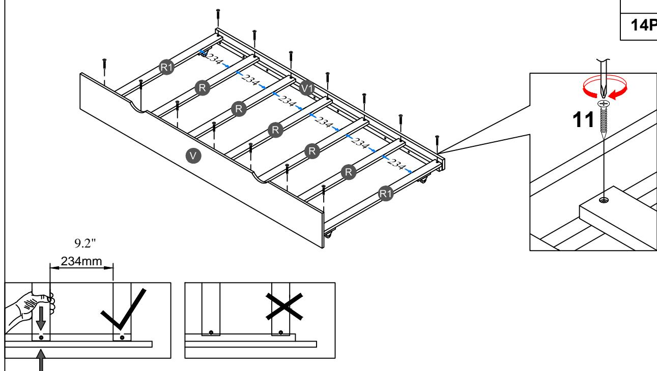
**NOTE:** Please make sure the bed slats close to the side rail before locking the screws to avoid breakage. This step is required for both the left and right sides. Moreover, please do not lock the screws of the bed slats at the outermost edge to avoid damaging.
