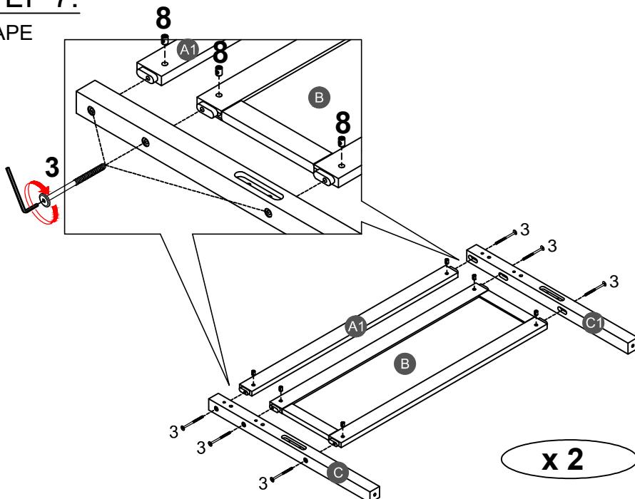
Note: Part 8 will face up with the "x" mark on it, otherwise it cannot be tightened
