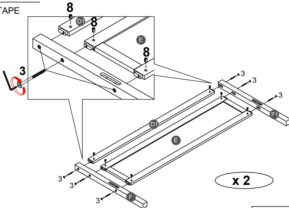
Note: Part 8 will face up with the "x" mark on it, otherwise it cannot be tightened
