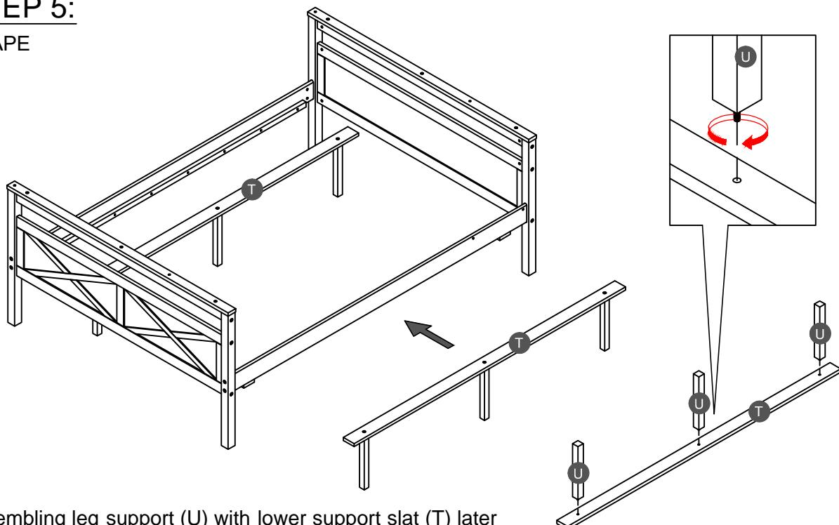
Assembling leg support (U) with lower support slat (T) later
