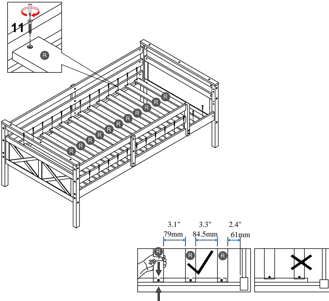
**NOTE:** Please make sure the bed slats close to the side rail before locking the screws to avoid breakage. This step is required for both the left and right sides. Moreover, please do not lock the screws of the bed slats at the outermost edge to avoid damaging.
