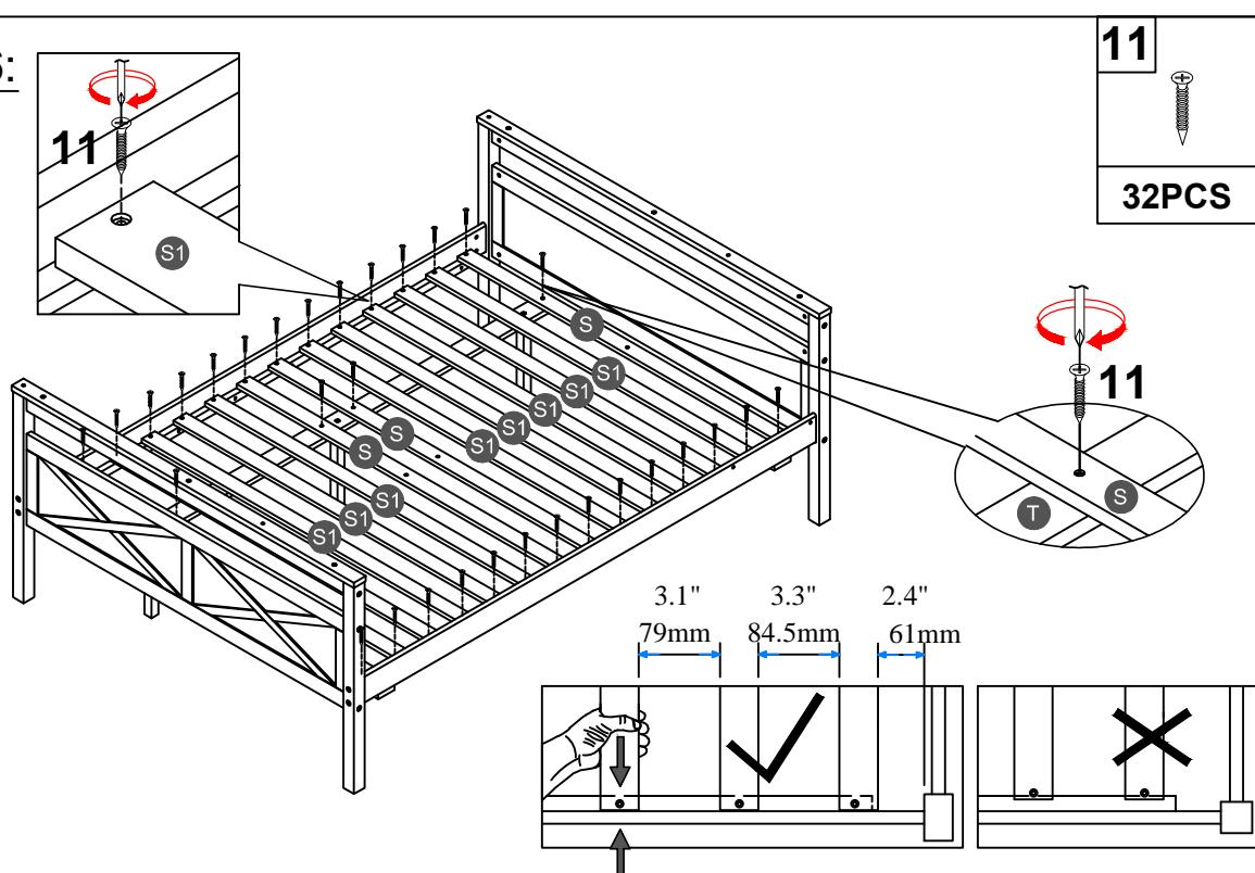
**NOTE:** Please make sure the bed slats close to the side rail before locking the screws to
