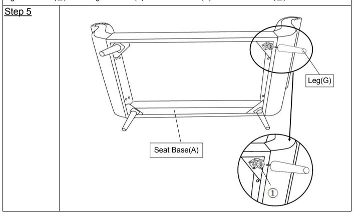
Install the Leg(G) into the bottom of Seat Base(A) by placing Plastic Washer(1) on the threaded stem. Then insert threaded stem into the threaded mounting postion at the bottom of Seat Base(A). Tighten by turning the Leg clockwise.
