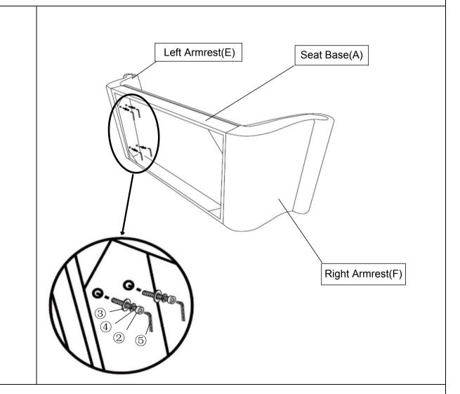
Attach the Left Armrest(E) to Seat Base(A) using Bolt(2), Spring Washer(4), Flat Washer(3), with Allen Wrench(5) and turning clockwise .
