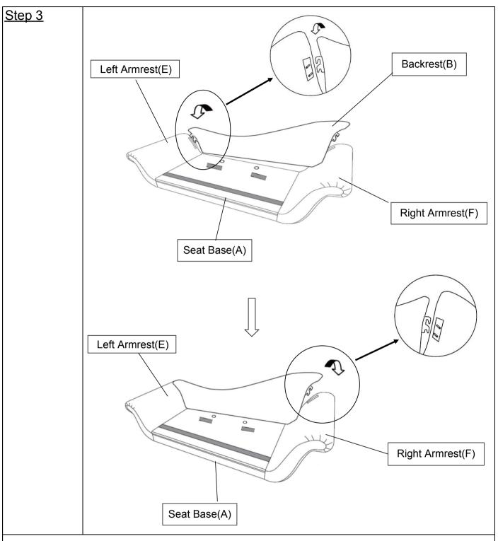
Standing behind the Seat Base(A) while holding Backrest(B). Hang on the hook of Backrest(B) onto the Preserved bolt of Left Armrest(E) as shown above, make sure two hooks are both on top of Preserved bolt
