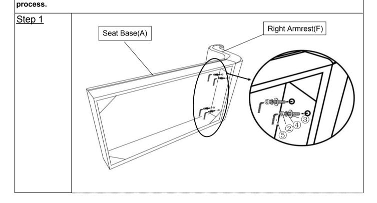
Open the carton and place all the parts on a clean, non-marring surface. Position Seat Base(A) as shown. Attach the Right Armrest(F) to Seat Base(A), using Bolt(②), Spring Washer(④), Flat Washer(③), with Allen Wrench(⑤) and turning clockwise. **DO NOT over tighten.**
