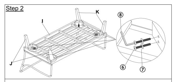
With assistance from your adult partner, place the Seat Frame (I) facedown onto a clean, non-marring surface, then attach the Right Leg(J) and Left Leg(K) to the Seat Frame (I) using the Bolts(6), Washers(7) and the Allen Wrench(8).
