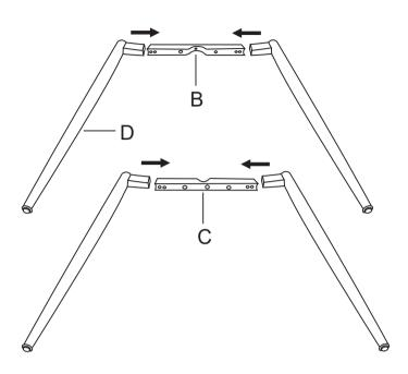
STEP 2 Attach the Legs (D) to Criss-Cross Supports (B&C) as shown in below diagram by using Allen Bolt (F) and Allen Wrench (J), Please tighten the bolts to 80%.
