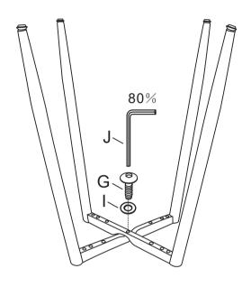
Attach the Criss-Cross Supports (B&C) to the swivel mech under the Seat (A) as shown in below diagram by using Allen Washer (I), Allen Bolt (H) and Allen Wrench (J), Please tighten the bolts to 80%.
