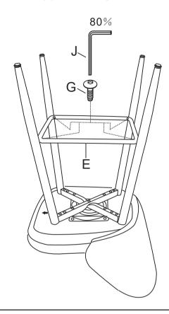
STEP 6 Use your body weight to adjust balance of this bar stool, then please 100% tighten all the bolts (F,G, H) all the way.
