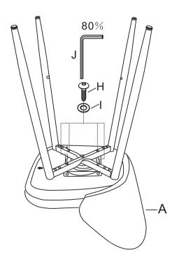
Attach the Footrest (E) to the Legs (D) as shown in below diagram by using Allen STEP 5 Bolt (G) and Allen Wrench (J), Please tighten the bolts to 80%.
