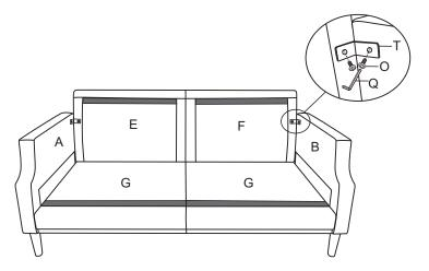
3.Connect the back frame (Part E&F) by aligning the metal piece (Part T) on Arms (Part A&B), then install Screw (Part O) with Toll (Part Q)
