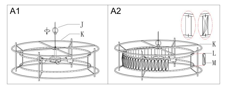
Step A1 » Screw loop (J) to the top of frame(K).
