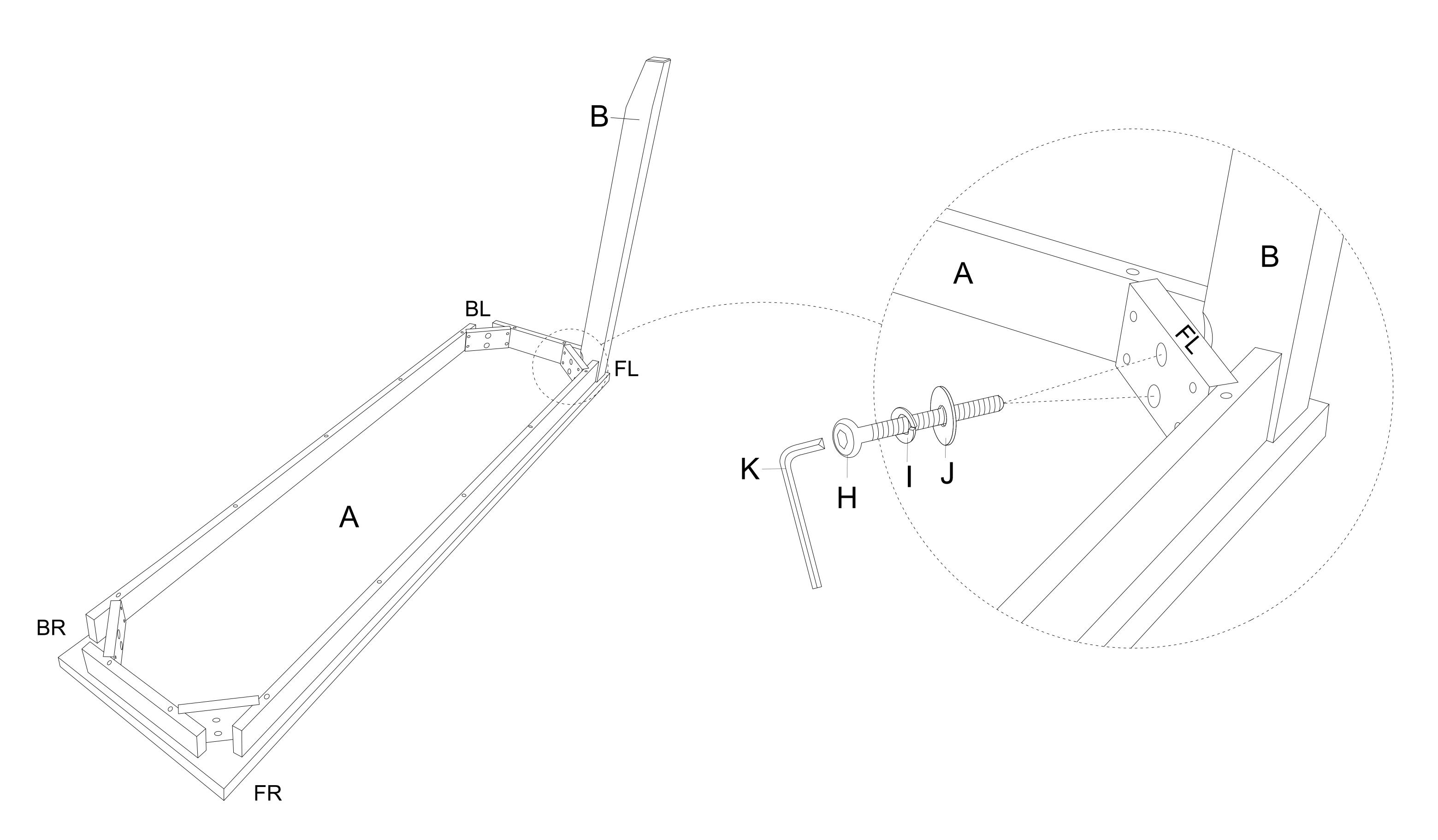
Attach the Table Leg BL (C) to the Table Top (A) using JCBC Bolt (H), Spring Washer (I) and Flat Washer (J) with the Allen Key (K). Before tightening the bolts, attach the Side Support (F) between the Table Leg (B & C).
