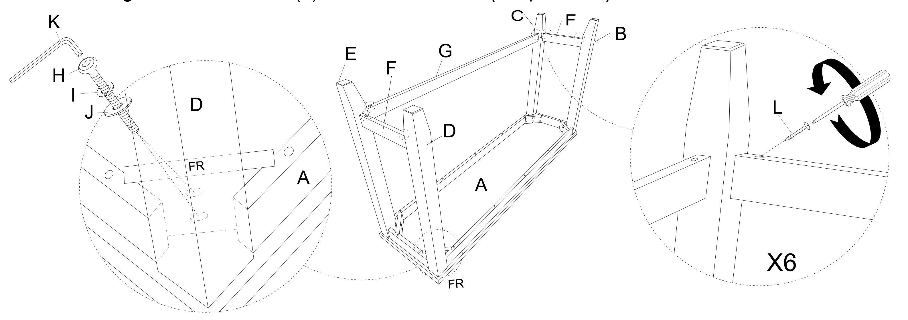
Stand the table on an even surface and check for balance. If the table wobbles slightly, apply downward pressure on the uneven leg and tighten all bolts to correct the imbalance. Once the table is balanced, apply downward pressure evenly in the center of the table and tighten all bolts, being careful not to over-tighten beyond the hole depth.
