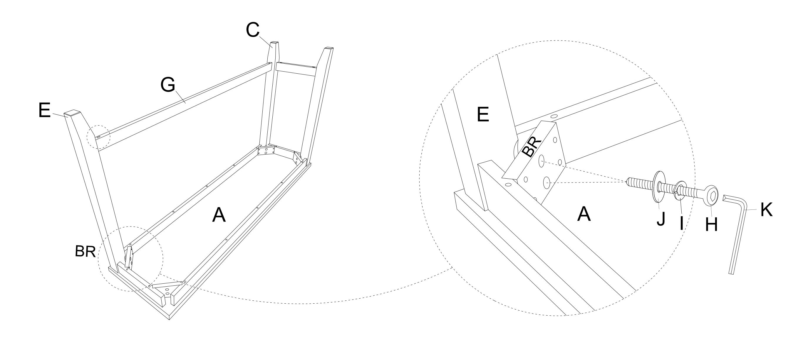
Attach the Table Leg FR (D) to the Table Top (A) using JCBC Bolt (H), Spring Washer (I) and Flat Washer (J) with the Allen Key (K). Before tightening the bolts, attach the Side Support (F) between the Table Leg (D & E). Finally, secure the Side Support (F) and the Cross Bar (G) using Pan Head Screw (L) with a screwdriver (not provided).
