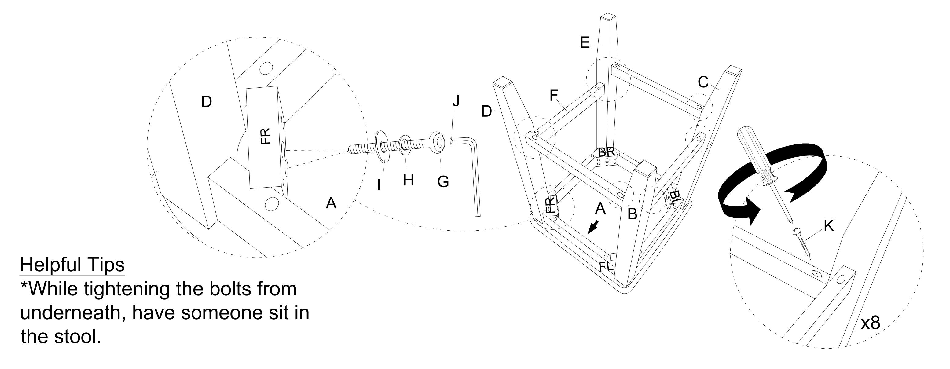
Stand the stool on an even surface and check for balance. If the stool wobbles slightly, apply downward pressure on the uneven leg and tighten the bolts to correct the imbalance. Once the stool is balanced, apply downward pressure evenly in the center of the stool and tighten all bolts, being careful not to over-tighten beyond the hole depth.
