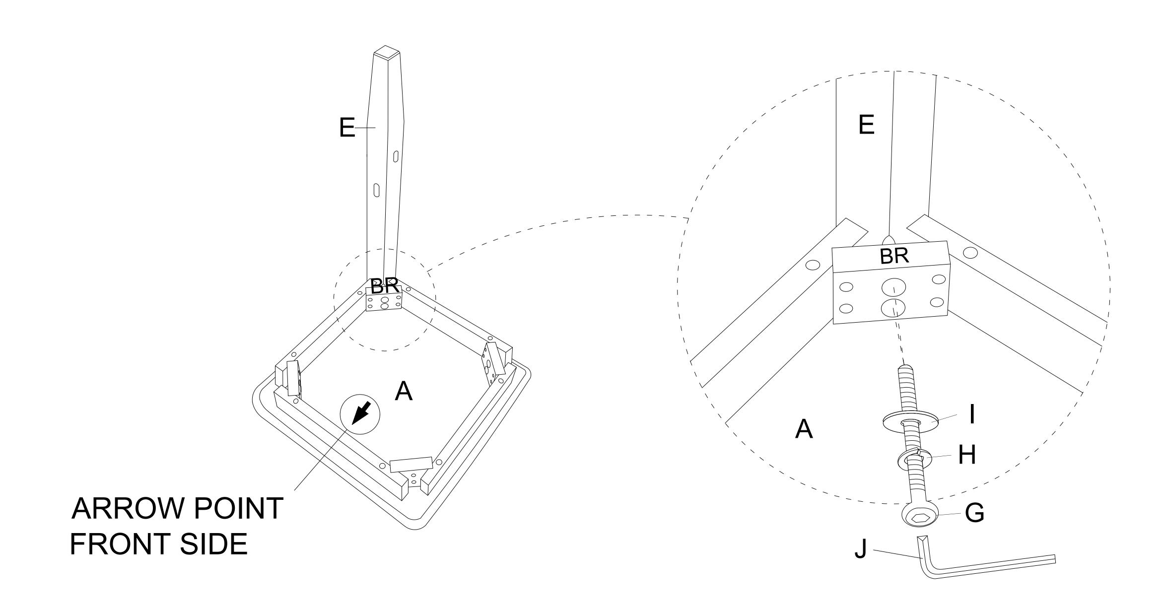
Take the Allen Key and turn the bolts until the legs are secured. DO NOT TIGHTEN THE BOLTS COMPLETELY.
