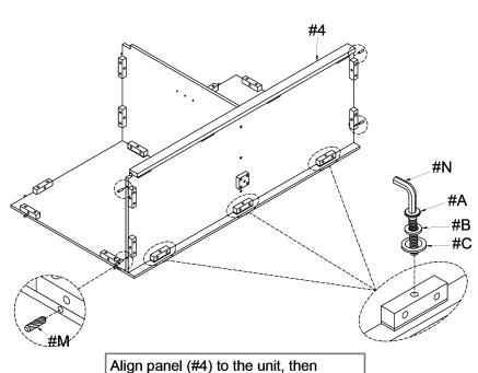
Align panel (#4) to the unit, then secure by using bolts (#A) with washers (#B,C). Insert dowels (#M) to panel (#4).
