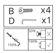
The screws in Step 1 and Step 2 must be tightened to 100% now.
