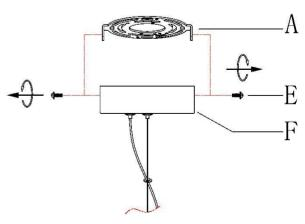
4 » Attach mounting plate (A) to the outlet box with mounting screws (D).
