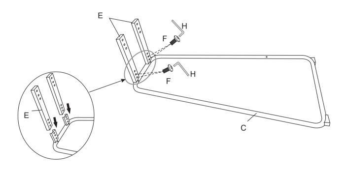
Attach Right Leg (D) to Leg Connecters (E) by using Bolt (F) and Allen Key (H) as STEP 2 shown in below diagram, please do tighten bolts 50%.
