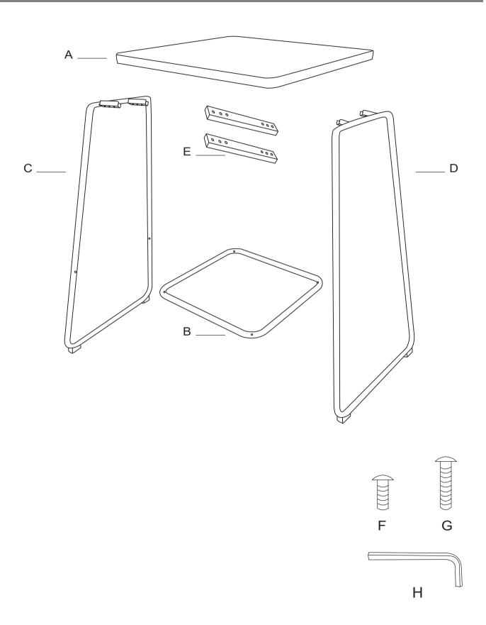
Attach Leg Connecters (E) to Left Leg (C) by using Bolt (F) and Allen Key (H) as STEP 1 shown in below diagram, please do tighten bolts 50%.
