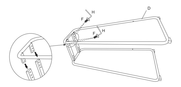
Attach Footrest (B) to Legs (C&D) by using Bolt (G) and Allen Key (H) as shown in below diagram, please do tighten bolts 50%. STEP 3
