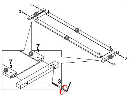
Note:Part 7 will face up with the "x" mark on it, otherwise it cannot be tightened
